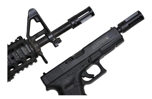
They have sufficient bore diameter to safely pass a .458 projectile, yet are tough enough to stand up to full auto fire from an 11.5" M16. They will outperform a military issue M4 flash hider in flash reduction. Slots to fit our wrenches are milled into the body.
